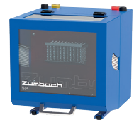
Spark Tester for cable insulations
