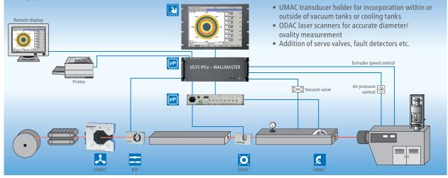
Wall Thickness Measurement and Control During the Extrusion of Pipe up to ø 620mm (24.41 in.) Transducer holders are available for measurement at the hot end or the cold end of the line. Optionally, also with integrated diameter measurement. At the hot end, the highest savings are possible:
