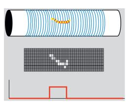
Our Rebar Software option allows the measurement of the characteristic dimensions of a Rebar product. It works within the standard PROFILEMASTER software during in-line production (hot or cold).
