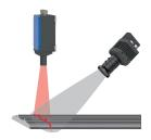
The measuring principle is based on 2D laser triangulation respectively light-sectioning technology. Four or more lasers illuminate the product surface and the associated matrix cameras capture the light contour from an oblique angle. A powerful and fast computer and the PROFILEMASTER software combine the captured segments into an orthogonal profile cross-section.
