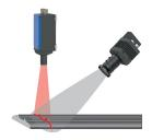
The measuring principle is based on 2D laser triangulation respectively light-sectioning technology. Four or more lasers illuminate the product surface and the associated matrix cameras capture the light contour from an oblique angle. A powerful and fast computer and the PROFILEMASTER software combine the captured segments into an orthogonal profile cross-section.
