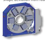
The mechanical concept and the basic elements are mostly the same as in the well proven oscillating gauges of the SMO series. Instead of power and signal transmission by a special cable solution, everything is now transmitted totally without contact. The rotating SMR models can be fitted with 1, 2 or 3 laser heads (axes). With 2 or even 3 heads, a full profile is generated after only 90 or 60 degrees respectively of the rotation. This means up to 10 full profiles/s.
