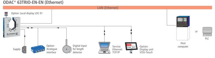
The built-in processor allows the acquisition and monitoring of the measured values, as well as statistic functions, parameter selection and many other functions. The EN version communicates via the integrated EN interface with a higher level system. The measured values and
