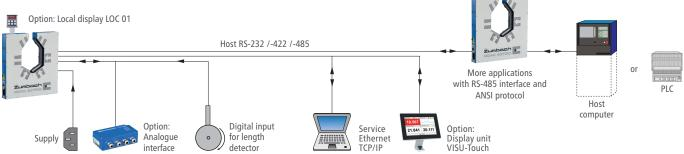
The built-in processor allows the acquisition and monitoring of the measured values, as well as statistic functions, parameter selection and many other functions. The RS version communicates via the integrated RS interface with a higher level system, like USYS from Zumbach, Host computer (or PLC). The Zumbach protocols ODAC or Host are selectable according to choice. The service interface (Ethernet TCP/IP) is used for configuring the measuring system.
