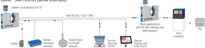
The built-in processor allows the acquisition and monitoring of the measured values, as well as statistic functions, parameter selection and many other functions. The RS version communicates via the integrated RS interface with a higher level system, like USYS from Zumbach, Host computer (or PLC). The Zumbach protocols ODAC or Host are selectable according to choice. The service interface (Ethernet TCP/IP) is used for configuring the measuring system.
