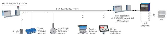
The built-in processor allows the acquisition and filtering of the measured values, as well as statistic functions, parameter selection and many other functions. The RS version communicates via the integrated RS interface with a higher level system, like USYS from ZUMBACH, host computer (or PLC). The ZUMBACH protocols ODAC, ASCII or the network capable ANSI software protocols are selectable according to choice.
