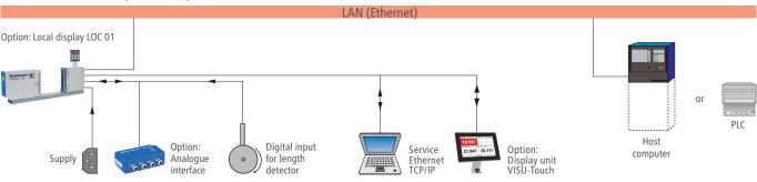
The built-in processor allows the acquisition and filtering of the measured values, as well as statistic functions, parameter selection and many other functions. The EN version communicates via the integrated EN interface with a higher level system. The selectable
