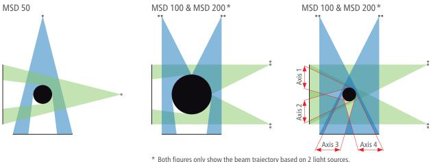
Both the MSD 100 and MSD 200 models are equipped with 4 light source pairs.
